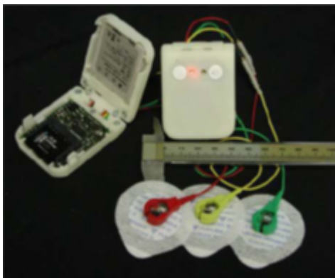
Fig. (2). Portable ECG recorder developed by Okada [3] Copyright © IEEE 2010.
