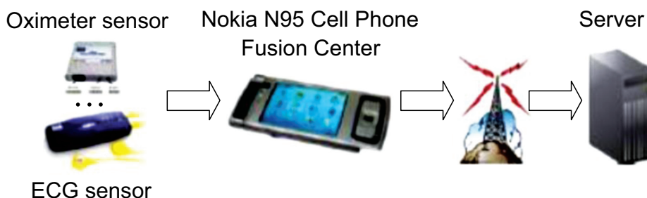
Fig. (8). KNOWME WBAN system [13,14] Copyright ©IEEE 2010.
