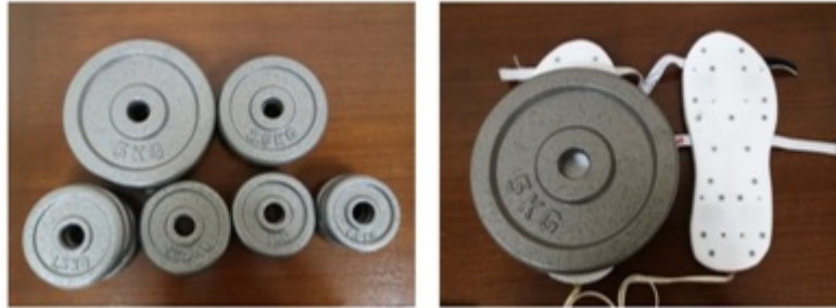
Fig. (4). Shows the accuracy test of WWSD with standard weights.
