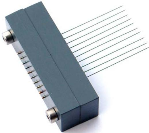
**Fig. (1).** Array of ten Viasys Healthcare Teca needles used for impedance measurements to produce a 2D invasive impedance tomogram.
