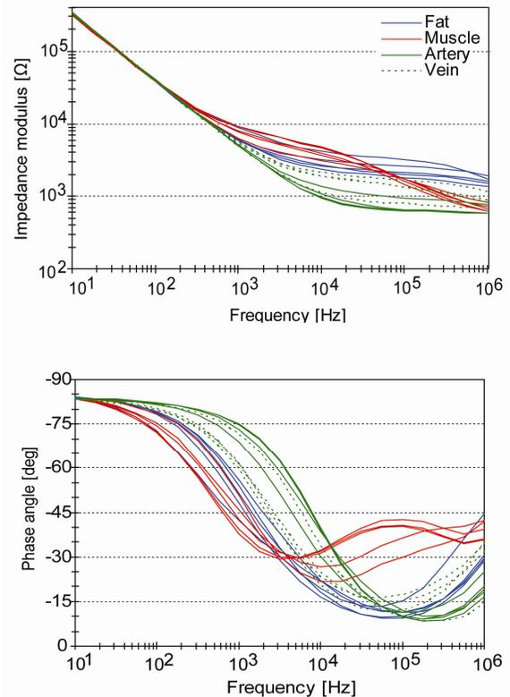
**Fig. (2).** Impedance spectra of Teca needles in different tissue types in an anesthetized pig.
