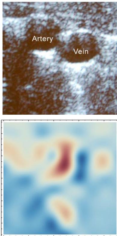
**Fig. (3).** Ultrasound image and plot of impedance phase angle at 316 kHz from approximately the same femoral area of an anesthetized pig, showing an artery and a vein. The phase angle ranges from 3.9 deg (red) to 49.7 deg (blue).
