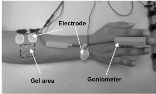
**Fig. (7).** The experimental setup for the tests of the effects of the ultrasound gel on the SEMG collection. The gel areas tested were 0, 1, 6, 10 and 24 cm<sup>2</sup> respectively.
