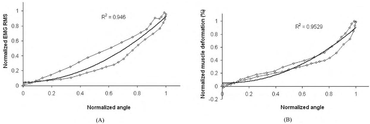
**Fig. (9).** The typical results of the second-order polynomial regression of different signals. (a) The regression result between the wrist angles and the RMS amplitudes; and (b) the regression result between the wrist angles and muscle deformations.
